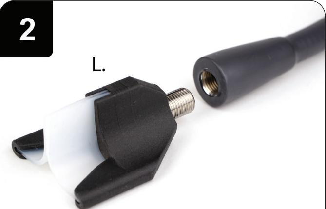
Thread **L** probe holder onto backplate arm
